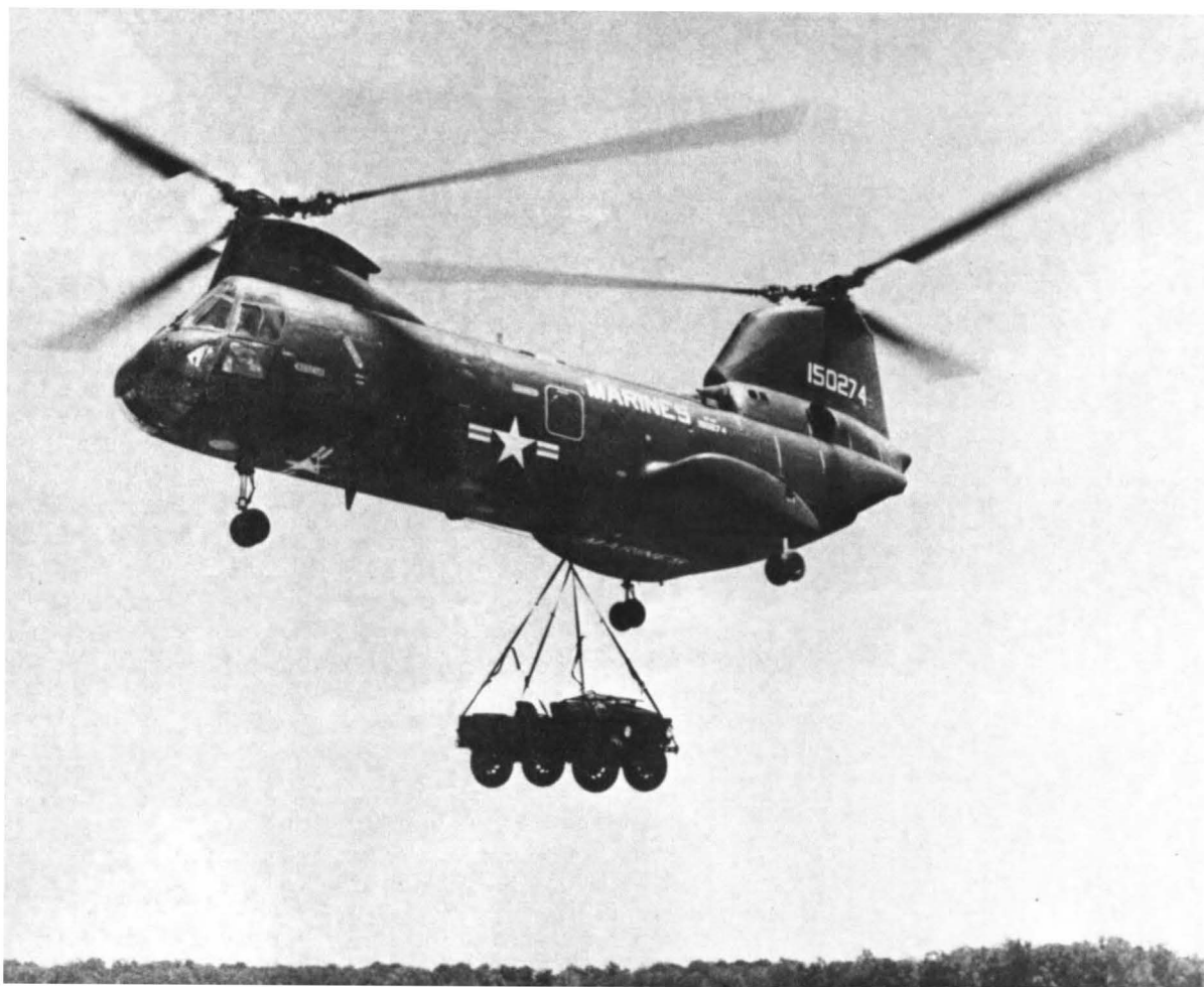
USMC Photo A411784 The CH-46A became the replacement for the UH-34. This aircraft is lifting a 1,780-pound "Mighty-Mite" vehicle on its 10,000-pound-capacity external cargo hook.
