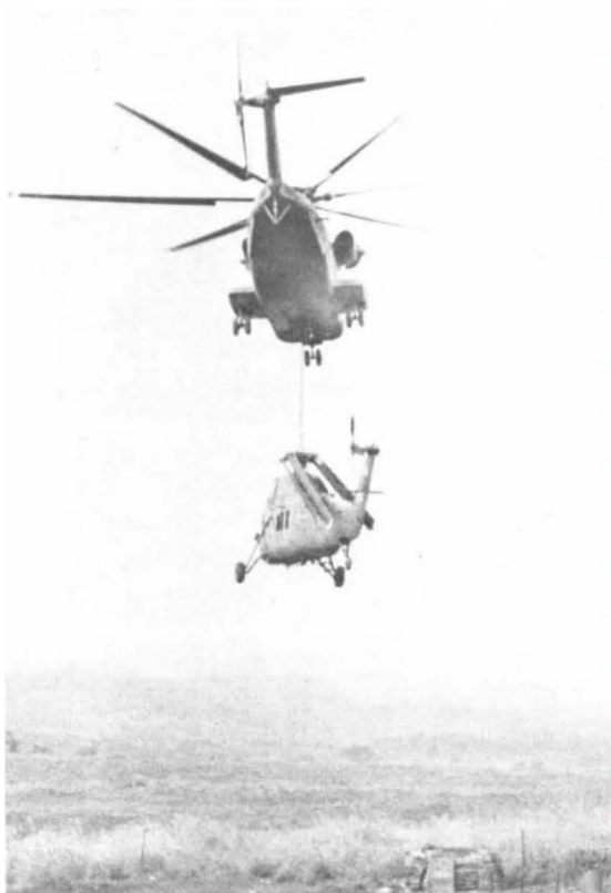
USMC Photo 3d-6-3471-67 A CH-53 lifts a disabled UH-34 out of Con Thien in northern I Corps in 1967. The CH-53A had enough power to lift a "Huss" with the rotor blades on.
